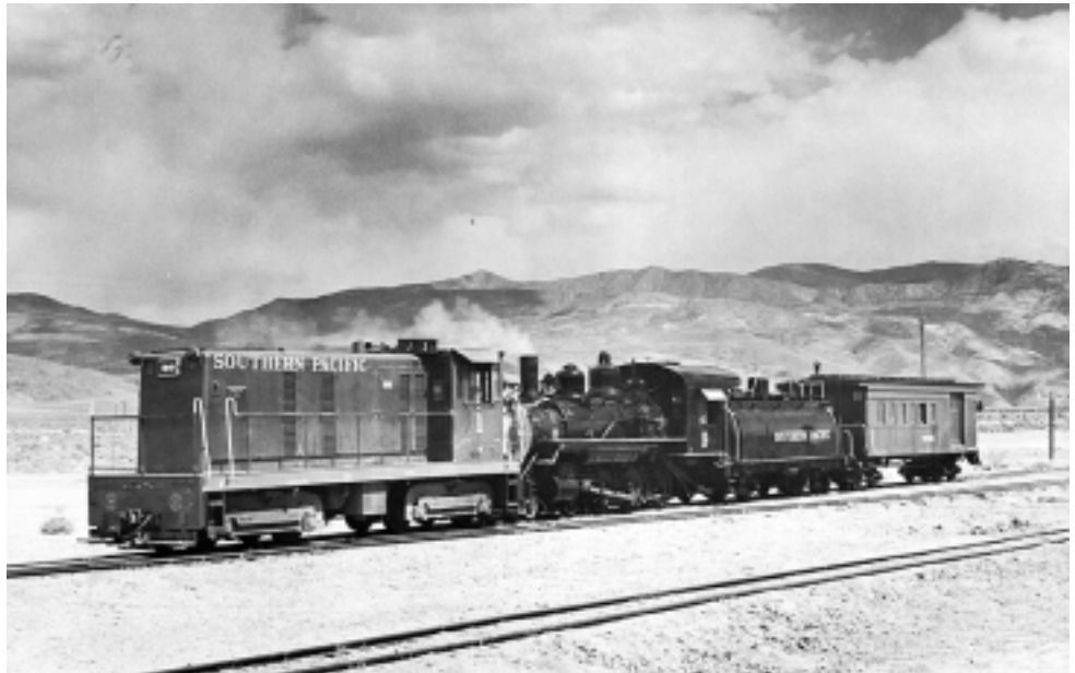
The "Grand Old Lady," engine No. 9, rides a free pass on her last trip. Having failed to pass an I.C.C. boiler inspection earlier, No. 9 was deprived of making her last run by her own power.
