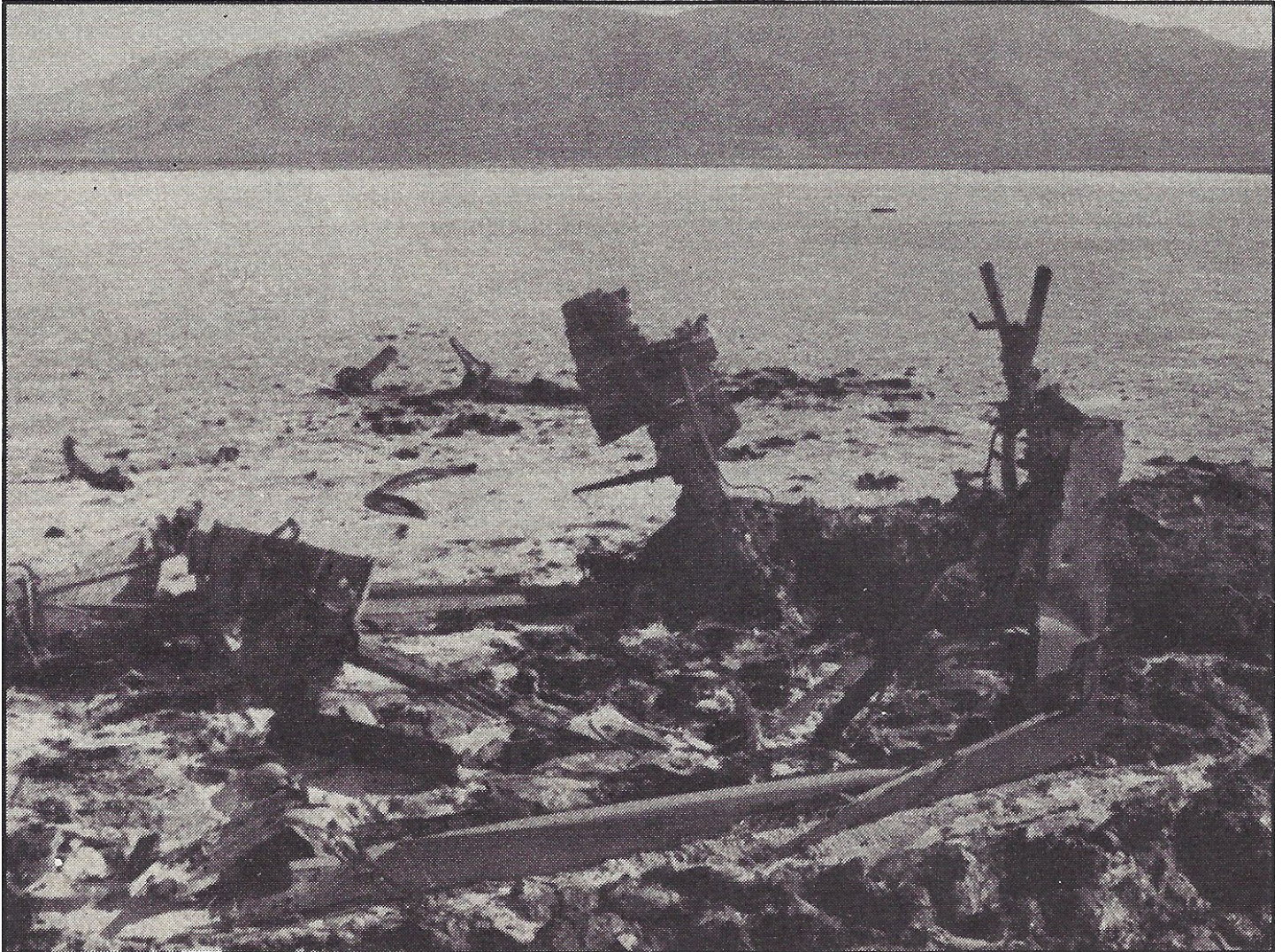
the remains of the TB-24J as it appears today. Scattered about the wreckage are the main landing gear struts, self-sealing rubberized gasoline tanks and various aluminum panels. Beneath the "V" strut is the nose gear with the tire still on the rim.
