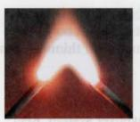
Early non-electric light sources for projectors used in 1860's included the oil lamp which emitted a very low brightness. In the 1880s, the incandescent lamps was pioneered by Edison and in the 1890's, the development of the carbon arc afforded the best natural-looking light source for both filming movies and projecting them. Projectors used carbon arc lamps until the late 1960s. "The length of those carbons for whatever reason was only twenty minutes which also dictated the
