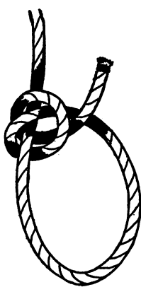
Midshipman's Hitch —A much better way of making the above, for the rope jams itself, and there is but little strain on the seizing. A man overboard catching a rope can make this—passing the bight between his legs and pressing the ropes together in his grasp in place of seizing. He could not tie a bowline or a noose unless he had slack.
