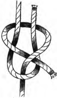
Single Sheet Bend —or Weaver's Knot, for joining ends of ropes together and without jamming, also to join one rope onto an eye splice
