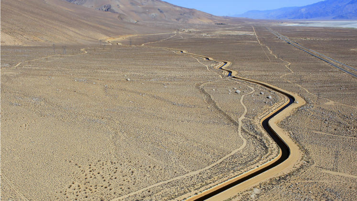
Aerial view of the Los Angeles Aqueduct as it flows south in its concrete-lined channel along Highway 395 in 2013. View is looking north into the Owens Valley. (Brian van der Brug / Los Angeles Times)
